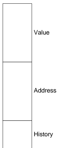
Figure 24 Structure of one internal buffer
